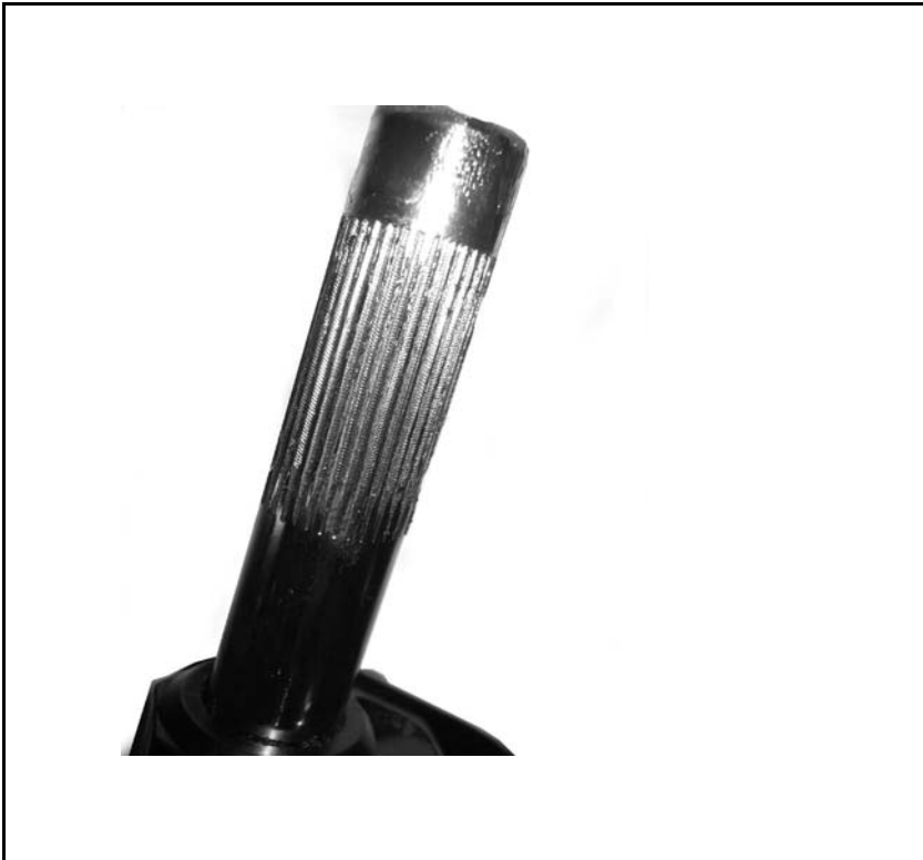
Foto from the steering column with the section with the knurling for the steering wheel hub (knurling according to DIN 82 - RAA1).
