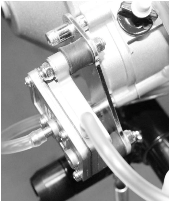
Foto of the frame with the section of the support for the fuel pump (fuel pump mounted)
