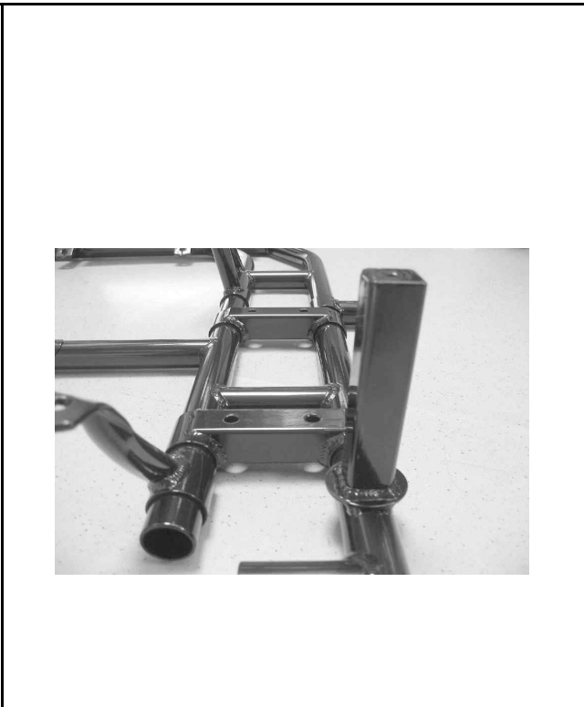
Foto of the frame from the back with the section of the support for the RTPS (Rear Tire Protection System)
