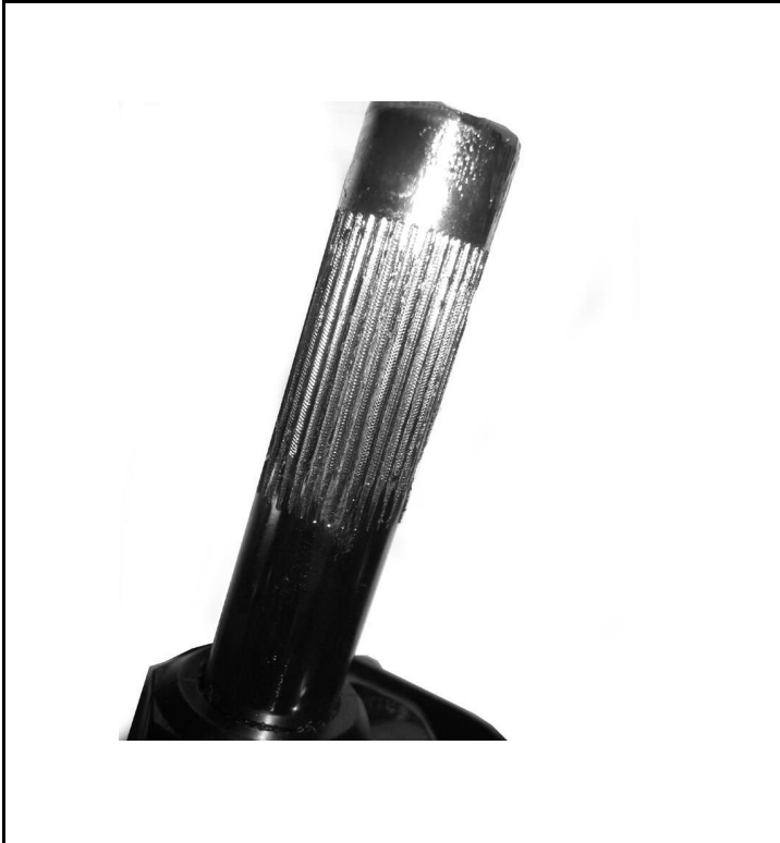
Foto from the steering column with the section with the knurling for the steering wheel hub (knurling according to DIN 82 - RAA1).
