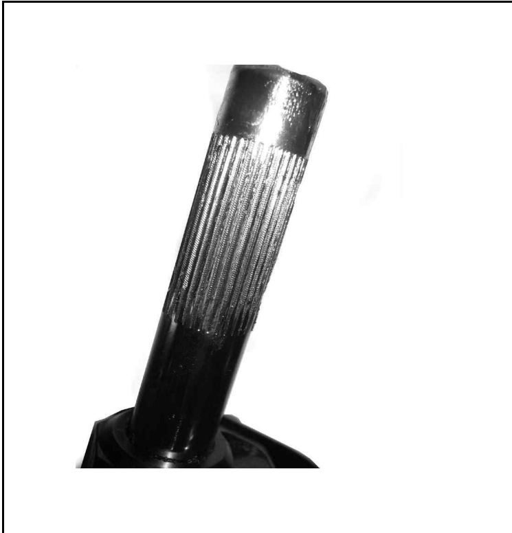
Foto from the steering column with the section with the knurling for the steering wheel hub (knurling according to DIN 82 - RAA1).
