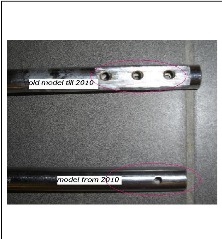
Photo from the steering column with the section with the knurling for the steering wheel hub (knurling according to DIN 82 - RAA1).
