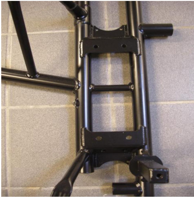
Photo from above of the frame with the section of the engine mount
