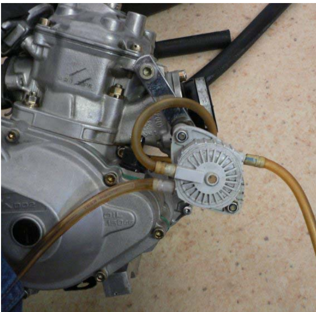
Photo of the frame with the section of the support for the fuel pump (fuel pump mounted)
