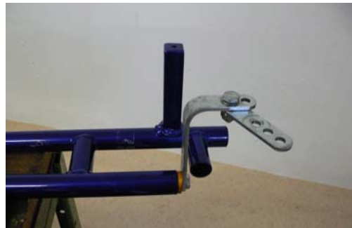
Photo from above of the frame with the section of the two supports for the exhaust system
