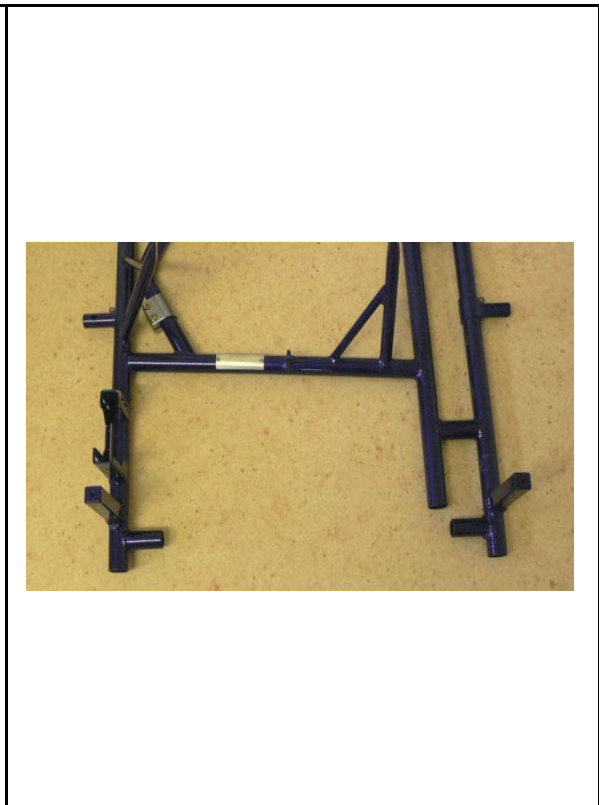
Photo from above of the frame with the section of the two supports for the RTPS (Rear Tire Protection System)
