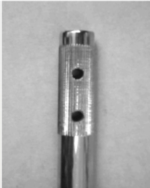
Photo from the steering column with the section with the knurling for the steering wheel hub (knurling according to DIN 82 - RAA1).
