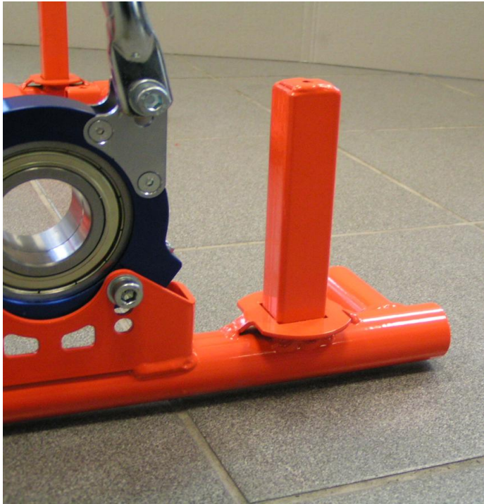
Photo of the frame from the side with the section of the support for the RTPS (Rear Tire Protection System)
