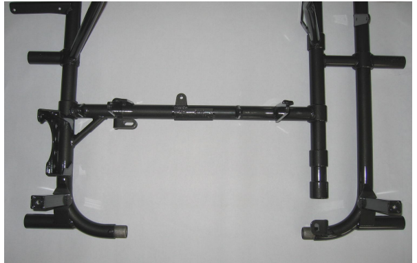
Photo from above of the frame with the section of the two supports for the RTPS (Rear Tire Protection System)
