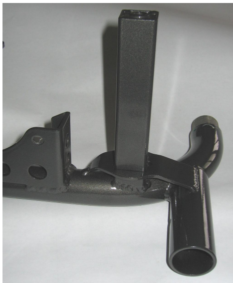
Photo of the frame from the side with the section of the support for the RTPS (Rear Tire Protection System)
