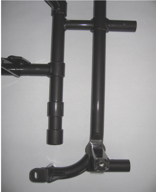
Photo from above of the frame with the section of the engine mount
