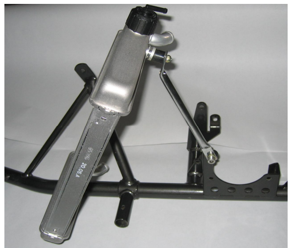
Photo of the frame from the side with the section of the supports for the radiator (radiator mounted)
