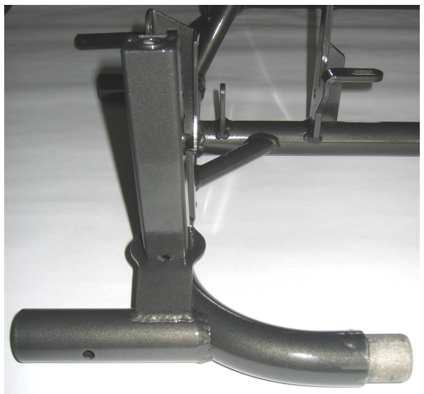
Photo of the frame from the back with the section of the support for the RTPS (Rear Tire Protection System)
