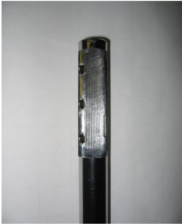
Photo from the steering column with the section with the knurling for the steering wheel hub (knurling according to DIN 82 - RAA1).
